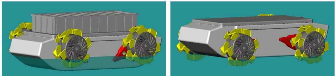
The system can adapt wheel height based on water level, vehicle load, or pitch changes due to acceleration and braking.
