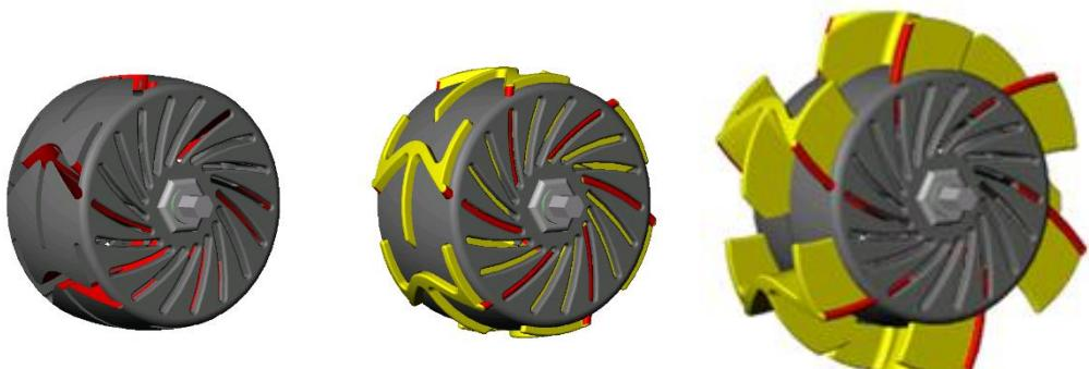
The tires are airless, built with soft, flexible spokes. This allows paddles to pass through the tread and nest between spokes without affecting the tire's flexibility or sealing - a major breakthrough.
