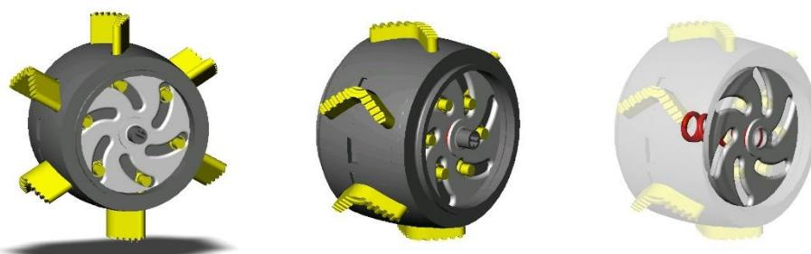
Paddles automatically retract on impact and redeploy when the obstacle is gone.
